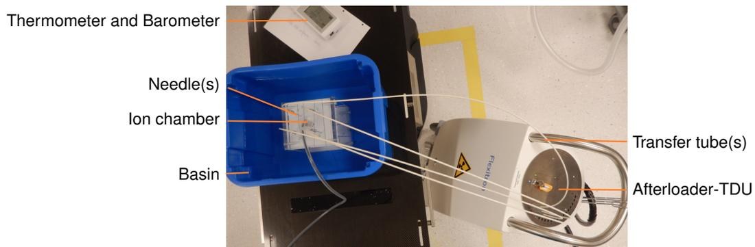
Figure 7: Measurement set-up with the 4 needle phantom.
