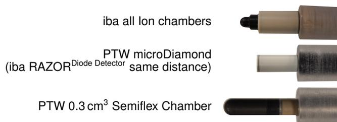
Figure 8: Indicator marks of the chambers when positioned in the fixing device.
